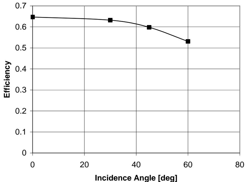
**Figure 1** Incidence angle modifier test: efficiency vs. incidence angle
