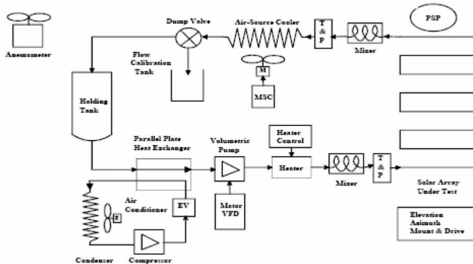
Figure 4 MATC solar collector test stand (closed loop), design by Thomas Kaminski
