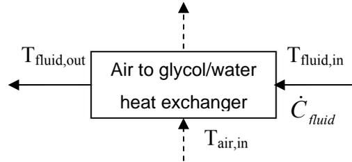
**Figure 6** Air to glycol/water heat exchanger
