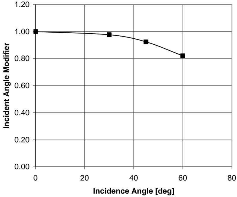
**Figure 2** Incidence angle modifier test: incidence angle modifier vs. incidence angle
