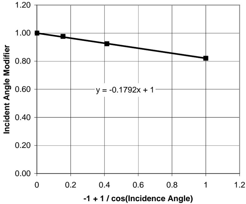
**Figure 3** Incidence angle modifier test: incidence angle modifier as linear function
