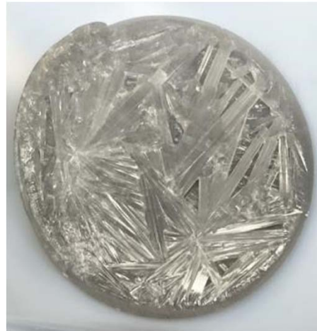
Pure Li_2BeF_4 (above) flows like water at 500°C (right)
