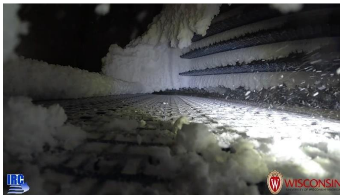
Figure 24: Frost buildup in a freezer captured by the Phantom’s camera on board the snowplow.
