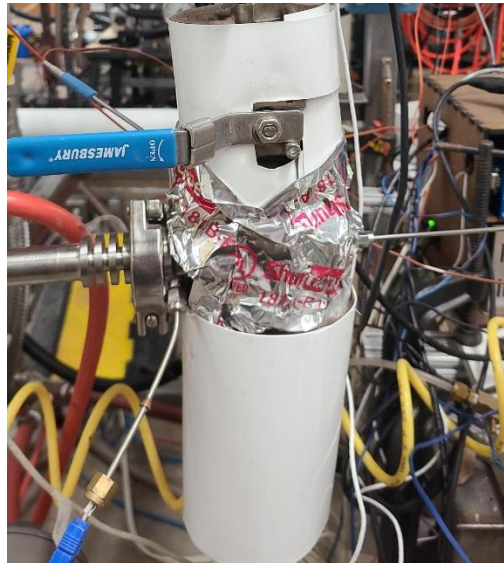
Figure F6: Insulated cross installed for the steam process parameter measurement as of December 2024.
