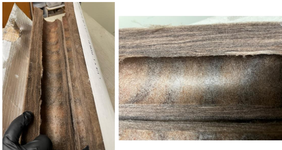
Figure F4: Photos of opened insulation after the initial runs with the new preheater (October 2024). The burns are only on the closest layer of insulation and don't extend further.
