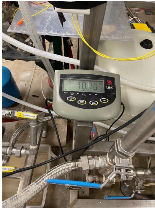
Figure A2: Photograph of the bladder tank scale readout.
