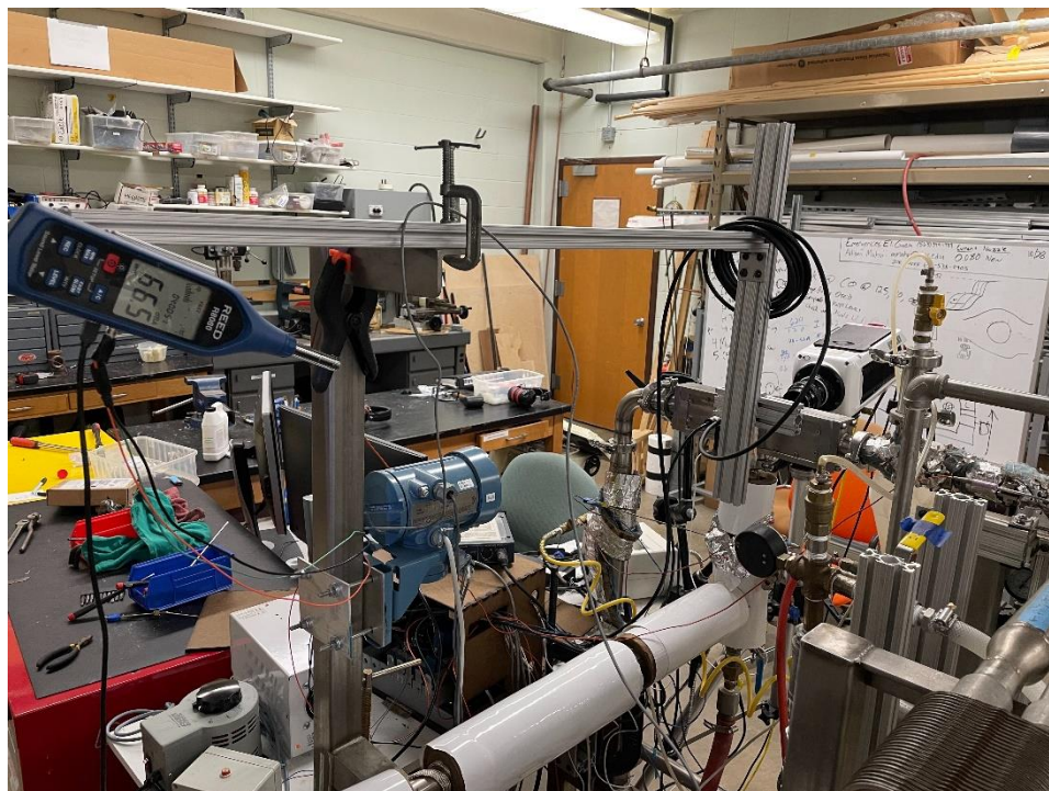
Figure C3: Boom arm to hold backlight and REED 8080 sound level meter.
