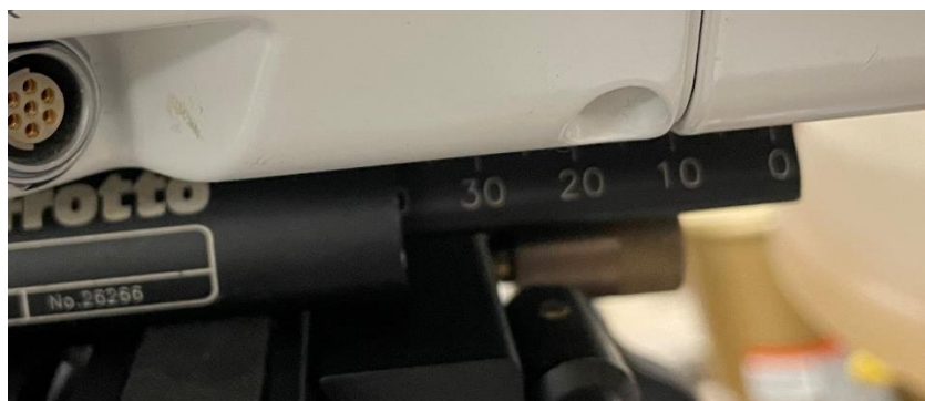
Figure C6: Dolly optical tray at its furthest setting as dictated by the set screw to attach it to the truck optical tray below it. Test videos are taken at a setting of 20 mm, then the camera moves forward for the reference image.
