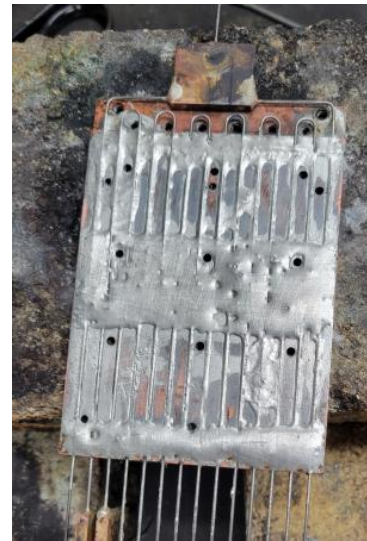
Figure 2.8. The condenser section, fabricated like the evaporator section, including a fill line.
