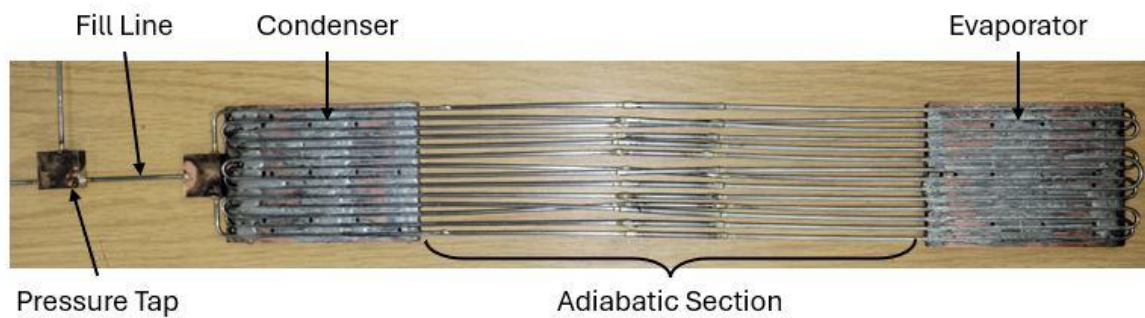
Figure 5.4. A picture of the HCPHP prototype specifying the locations of the fill line, pressure tap, and the three standard heat pipe sections.
