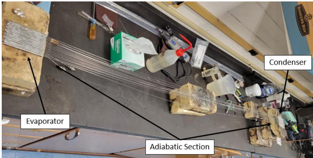
Figure 2.9. A picture of the 1.75 m PHP, demonstrating its very large length/width ratio.
