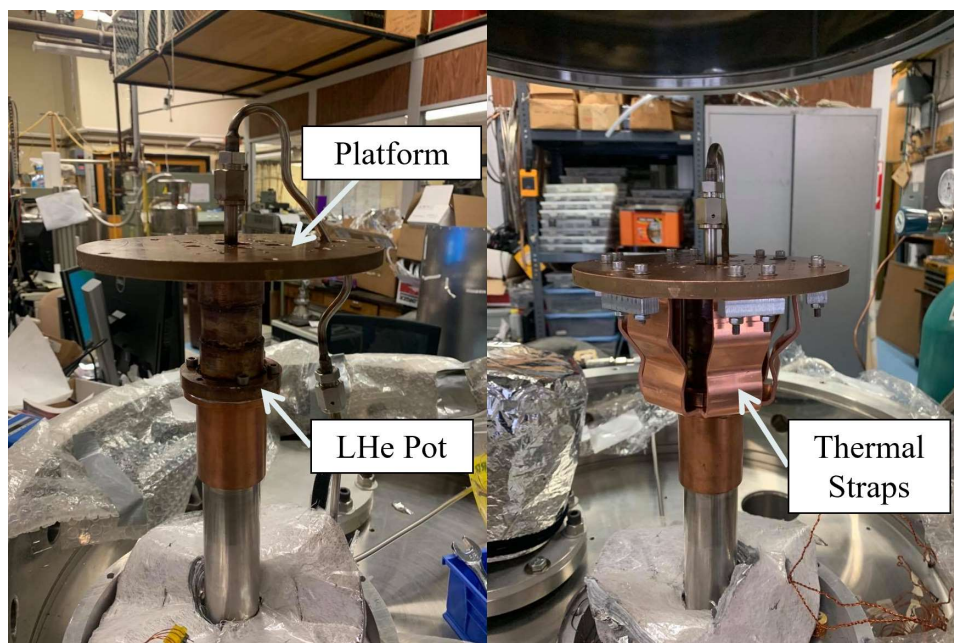
Figure 2-7. Final liquid helium pot configuration.
