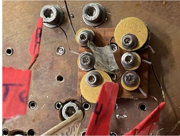
Figure 2-10. Copper plate mounting surface used for temperature sensor calibration.
