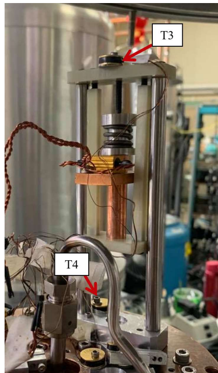
Figure 4-6. Test fixture for fixture resistance determination.
