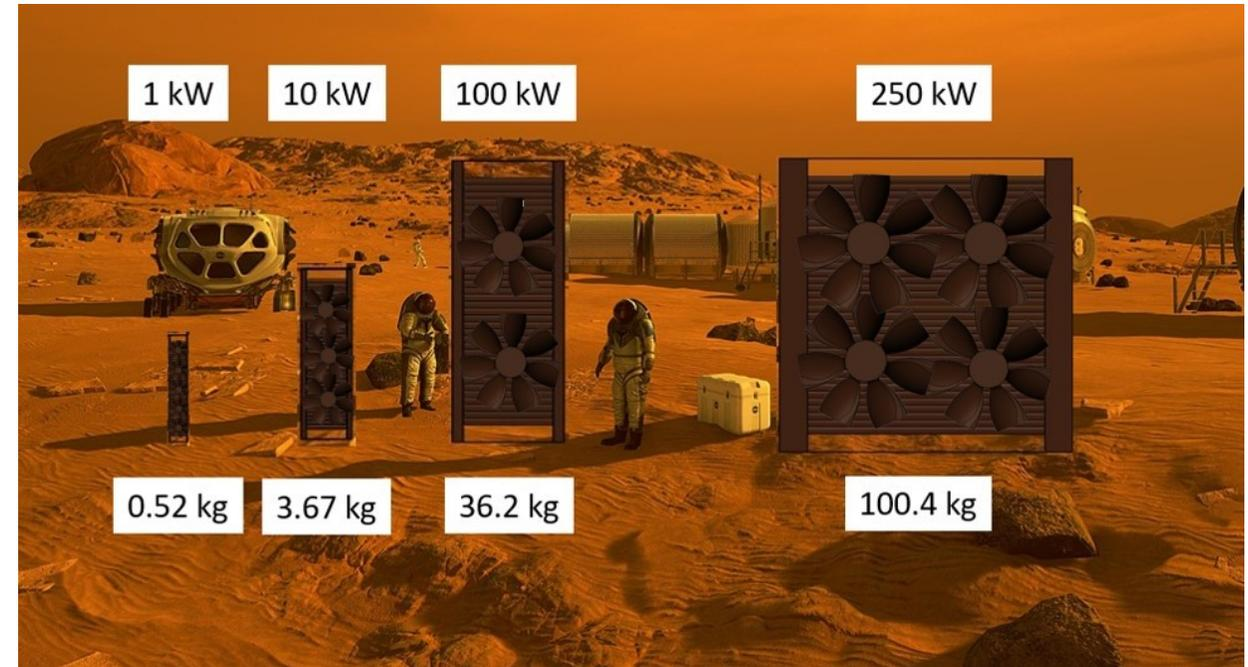
Illustration of heat exchangers optimized for various heat rejection loads. Background image credit: NASA
