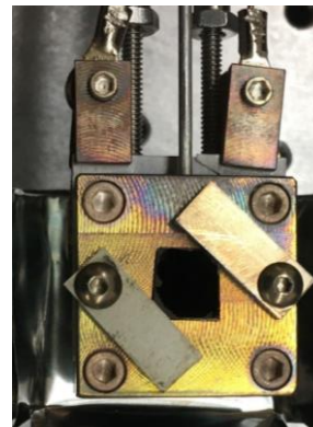
(left) Reference sample and (right) CNT mounted on heater
