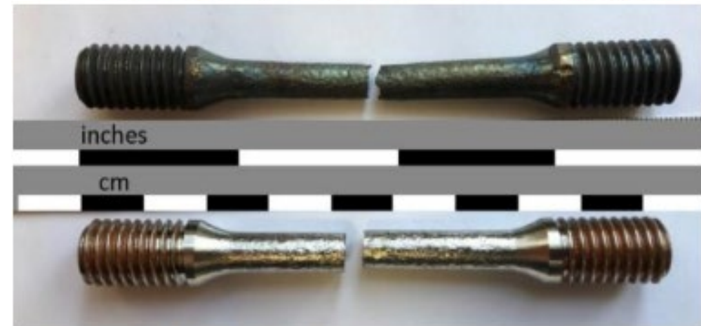
Figure 11: Alloy 617 diffusion-bonded samples tested at room temperature (bottom) and 750°C (Top)
