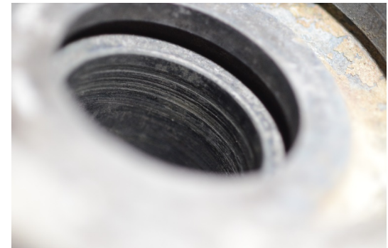
Stage sleeve and bushing with evidence of galling & rubbing post molten salt testing.
