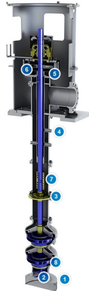
Sulzer VEY Pump design cross section
