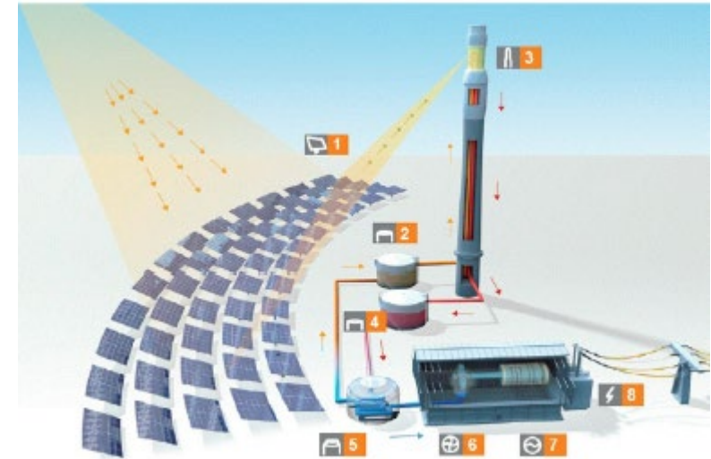
(1) solar field, (2) cold salt tank, (3) tower with receiver, (4) hot salt tank, (5) steam generator, (6) steam turbine, (7) electric generator, (8) electrical transformer.
